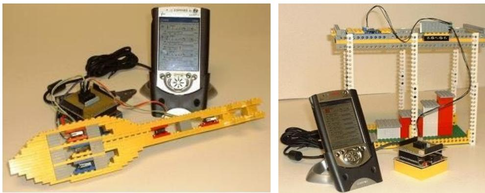
*Figure 14: MICK musical instrument construction kit. Left: a guitar with switches. Right: a sliding car with a light sensor.*
