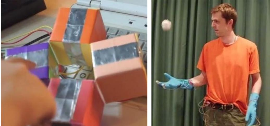
*Figure 10: Invented object-scale instruments. Left: Marimba Cubes that play individual notes when touched, or chords when folded together. Right: Beat Balls is a juggling system that triggers a note each time a ball is caught or thrown.*
