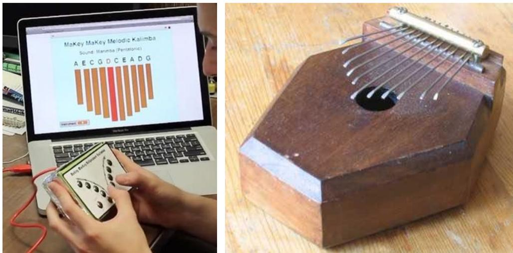
*Figure 14: A reconfigurable kalimba. Left: The kalimba's notes are triggered by tapping metal tabs with the thumbs. A Scratch project shows its current pitch arrangement. Right: an acoustic kalimba, played by plucking tines in a similar vee shaped arrangement.*
