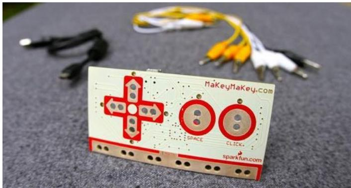
*Figure 10: the MaKey MaKey circuit board.*
