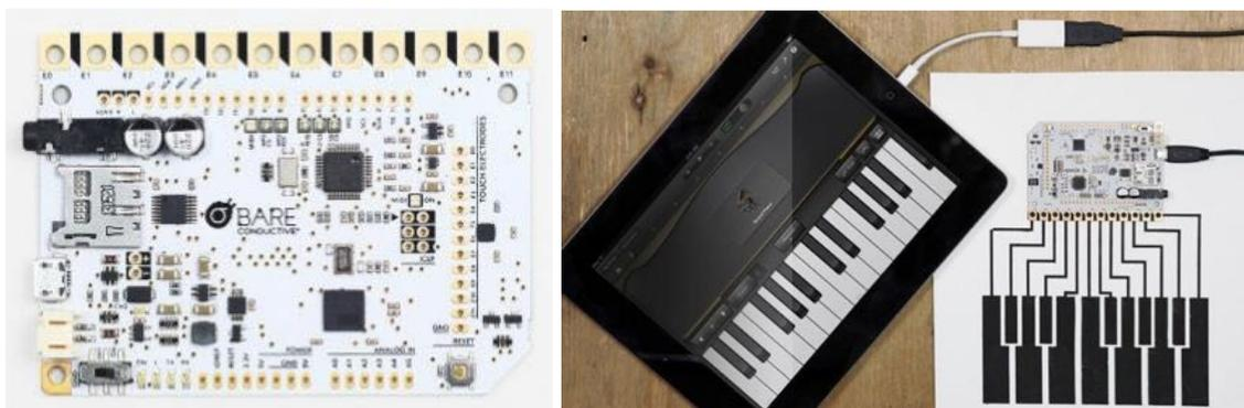
Figure 17: The TouchBoard sensor board. Left: the circuit board, with 12 capacitance sensing inputs along the top. Right: TouchBoard connected to a painted piano to control an iPad music app (images by Bare Conductive).
