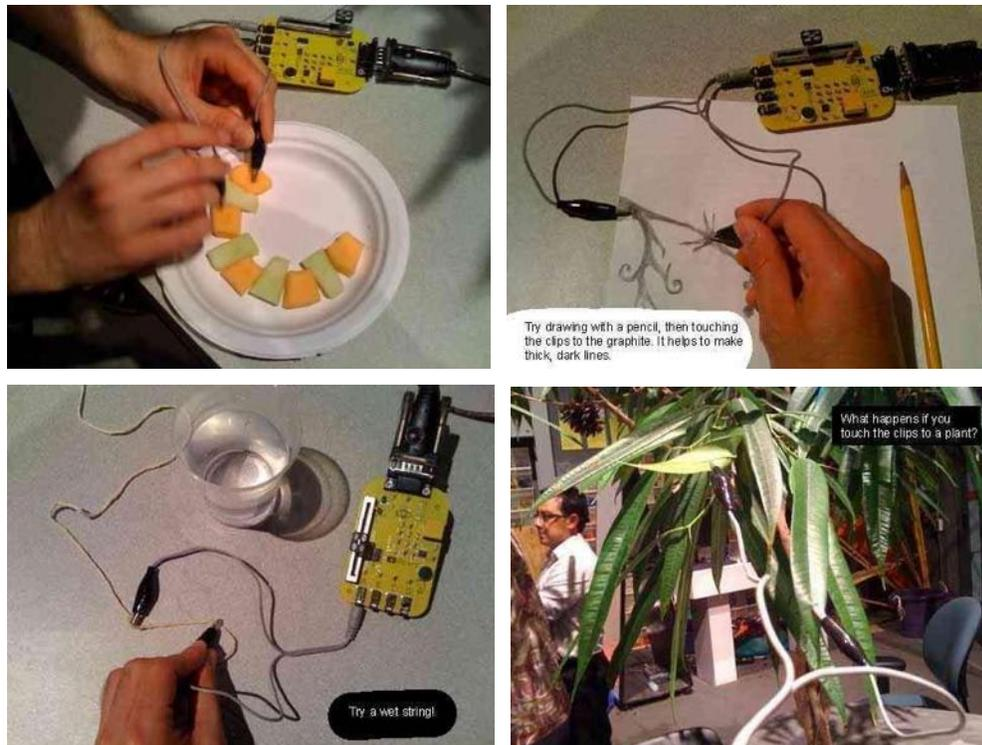
Figure 5: Scratch Sensor Board musical instruments. Top left: a melon piano. Top right: a musical pencil drawing. Bottom left: A wet string instrument. Bottom right: musical leaves.
