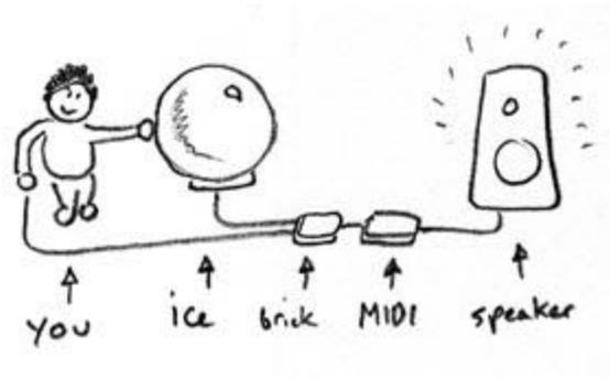
Figure 4: The “Ice Theremin.” Left: a child plays with a version of the instrument, completing a circuit to generate sound by touching a foil-tipped wand to a ball of ice. Right: my diagram showing the parts of this resistance sensing instrument, including the Cricket programmable brick.
