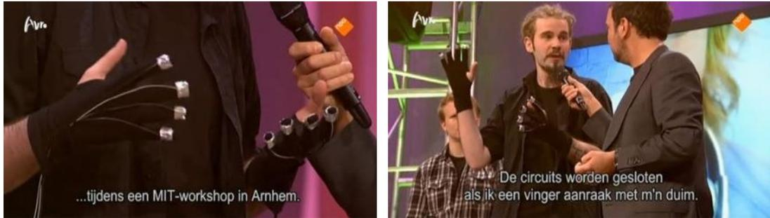
*Figure 25: The musical gloves on Dutch television. Right: the translation of the full sentence he says is “I invented them during an MIT workshop in Arnhem.” Right: the caption translates to “the circuits are closed when I touch a finger with my thumb.”*
