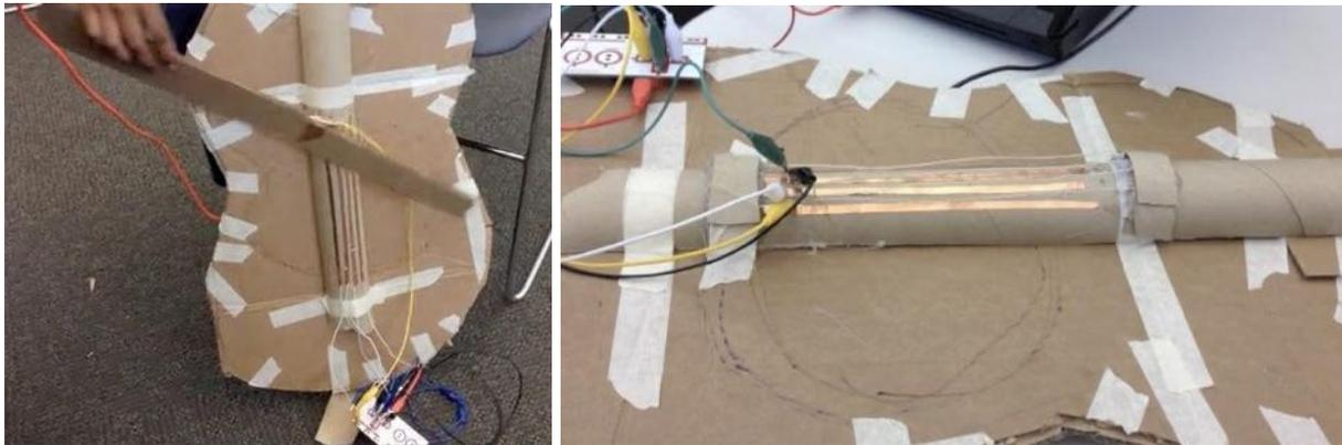
*Figure 29: Two iterations of Ben’s cello. Left: an earlier version played by touch a grounded bow to strips of conductive tape on a tube. Right: a later version with a bridge that supports wires acting as strings that trigger notes when pressed against the tape strips.*
